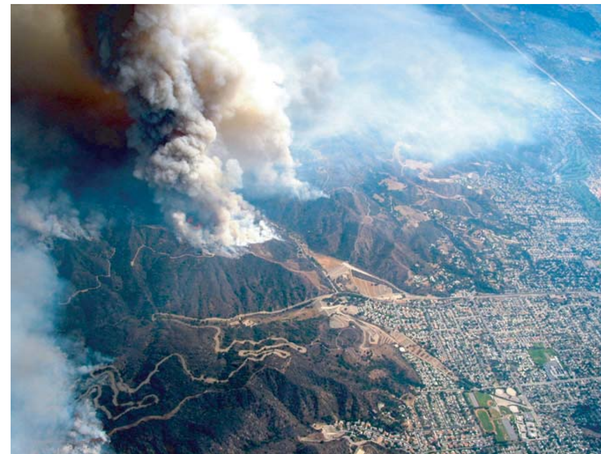
Urban development near wildland areas introduces many natural hazards including fire-related debris flows. Fires in wildland areas greatly increase the debris-flow hazard. Brief intense thunderstorm rainfall of 0.5 inch or less can trigger debris flows in burn areas (U.S. Forest Service photo).
