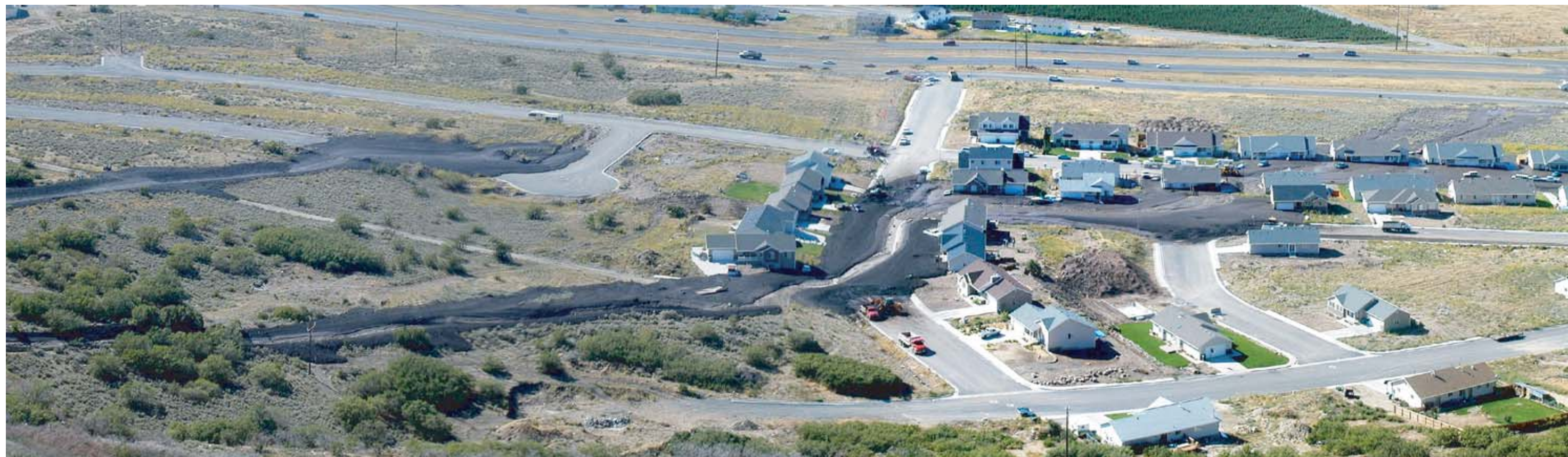
Oblique air photo showing debris-flow deposits from the September 12, 2002 event. Three debris flows deposited sediment in subdivisions built on alluvial fans in Spring Lake and Santaquin, and others deposited sediment in undeveloped areas. The debris flow shown above partially buried several vehicles, broke through a house wall, and entered other houses by breaking basement windows and doors. Five homes and two businesses received major damage and 27 homes received minor damage (U.S. Forest Service photo).
