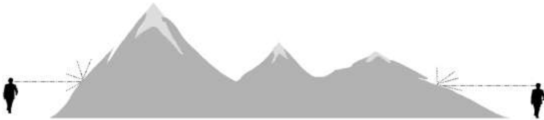
Line of sight path is broken
