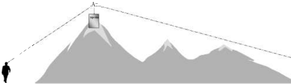
Repeater to provide line of sight
