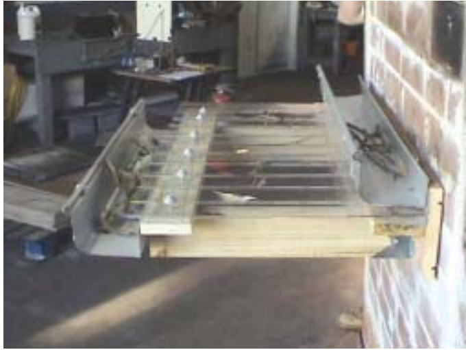
Laserlite clad timber framed pergola construction with typical accumulated debris including leaves and bracken ready for bushfire fire testing.
