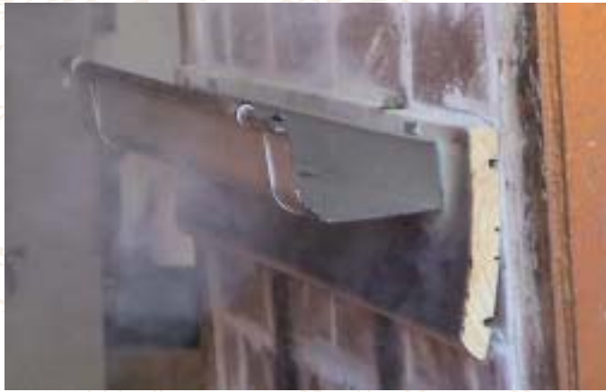
Experimental indicative bushfire fire test on a non fire retardant treated timber fascia / gutter assembly in the early stages of radiant heat exposure
