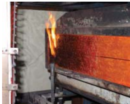
Alsynite Paraphen® phenolic sheet material being subjected to stringent spread of flame testing with radiant heat source and simultaneous pilot flame
