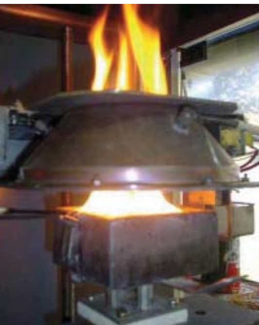
Cone calorimeter test to AS/NZS3837 on non fire retardant timber showing extensive flaming and significant heat release rate
