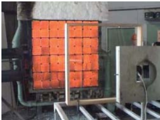
Timber framed window assembly during indicative bushfire fire testing. Note - Radiometer in foreground and radiant heat panel in background.
