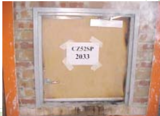
Picture showing a pilot scale fire resistance test on a fire door incorporating a Lorient Integrity® automatic door seal
