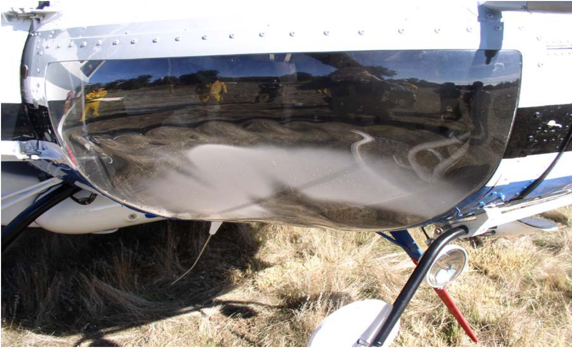
Right Seat Chin Bubble Damage
