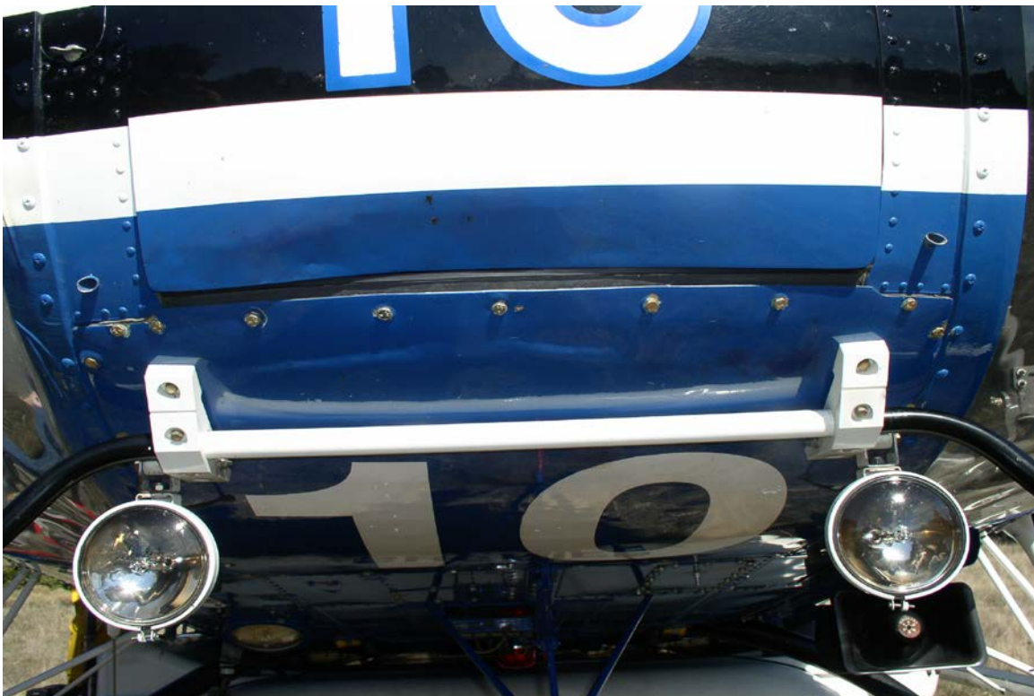
Nose and Battery Door Damage
