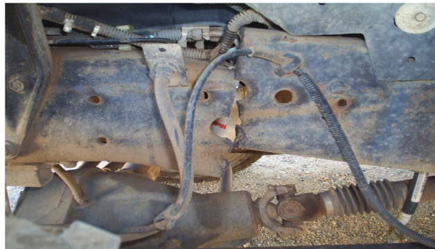
Picture 3: Broken Frame on Drivers Side
