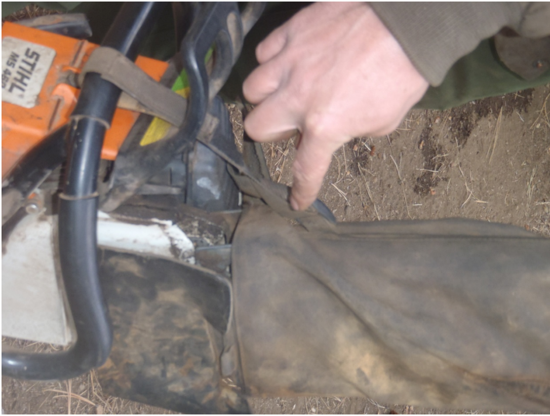
Photo of dawgs properly wrapped. Notice the leather flaps do not effectively cover the outermost dawgs.
