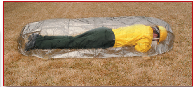
Figure 3—This firefighter, who is 6 feet 2 inches tall and weighs 235 pounds, will find the large fire shelter roomier than the regular shelter. The photo has been digitally altered to show the firefighter as though the shelter was transparent.
