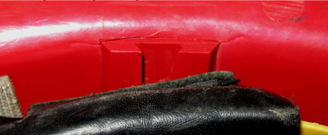
Figure 3 – Damage to shell, right rear suspension attachment area
