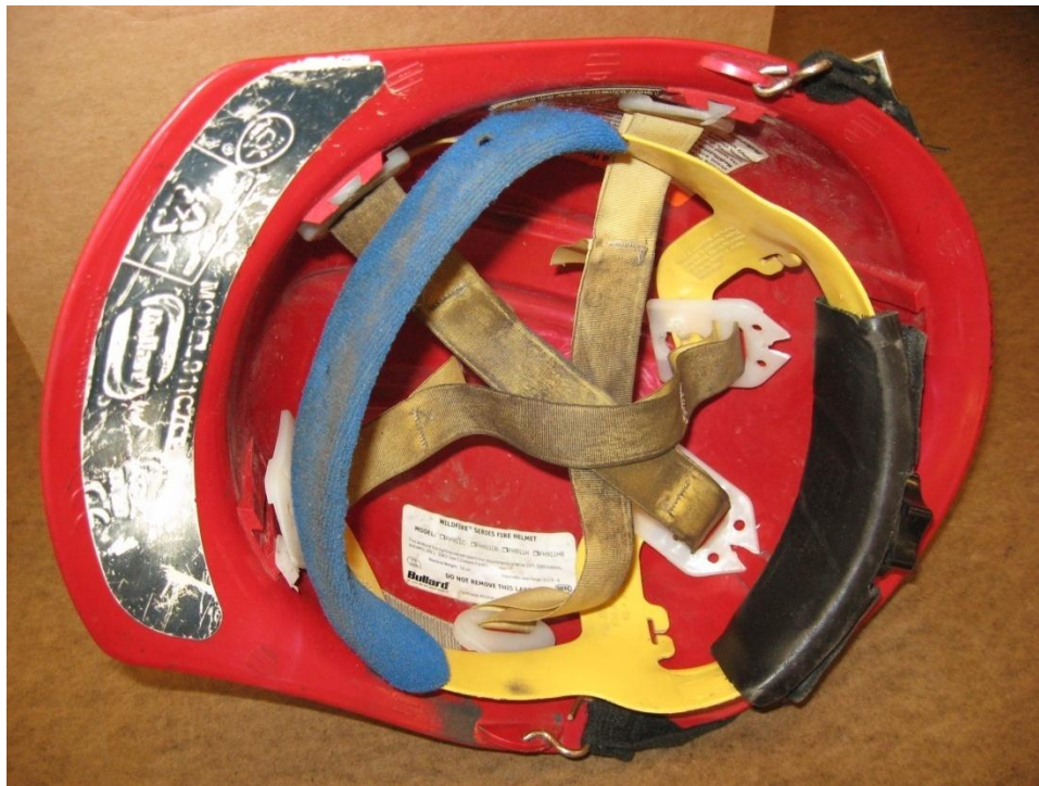
Figure 2 – Condition of inside of hardhat
