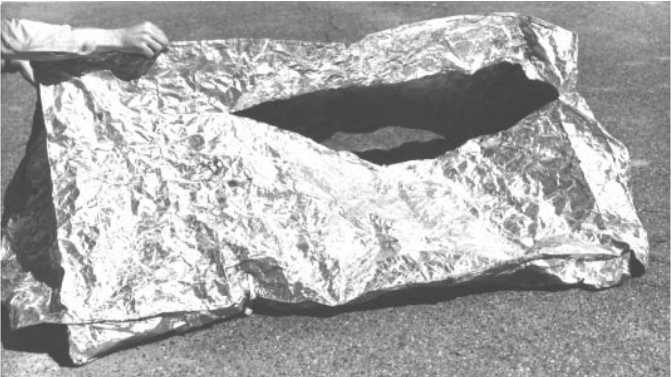
Figure 2.—Even a damaged fire shelter provided protection for two entrapped firefighters.
