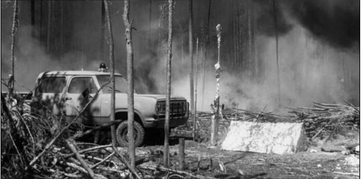
These vehicle entrapment tests in Dillon, MT, provided field comparisons of the effects of heat on fire shelters and engines.
