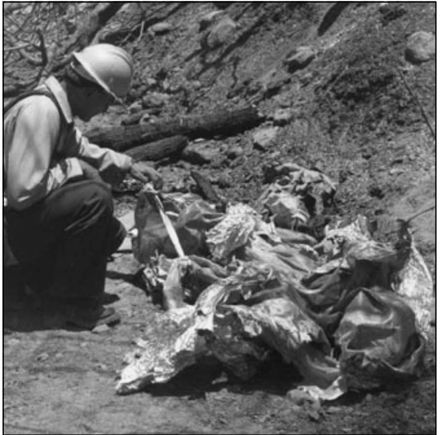
Close inspection of the fire shelter provides clues of temperature ranges experienced during an entrapment.
