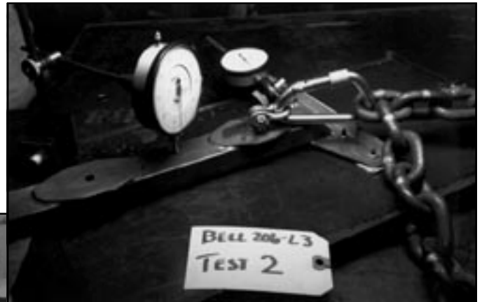
Applying stress to the anchor plate for a Bell 206-L3 helicopter.
