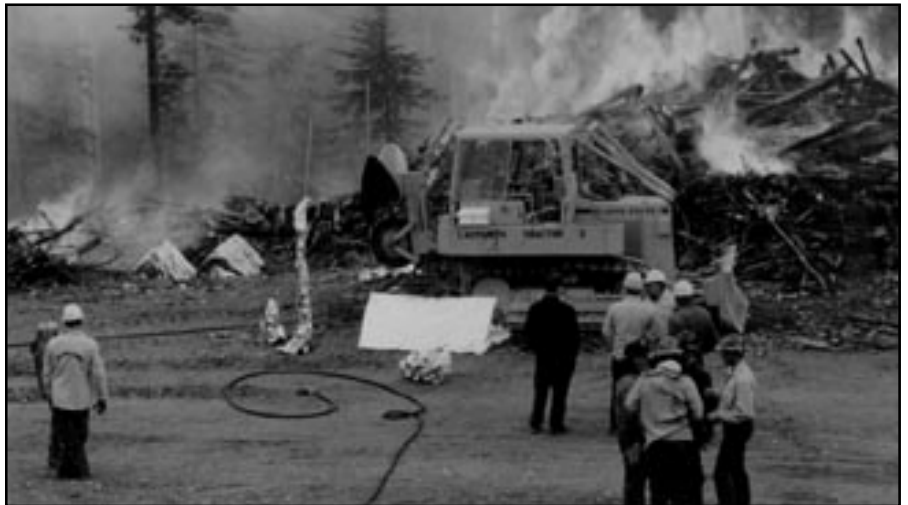
This field test considered the effects of sprinklers inside the dozer's rollover cage. The sprinklers were designed to protect the operator if a fire burns over.
