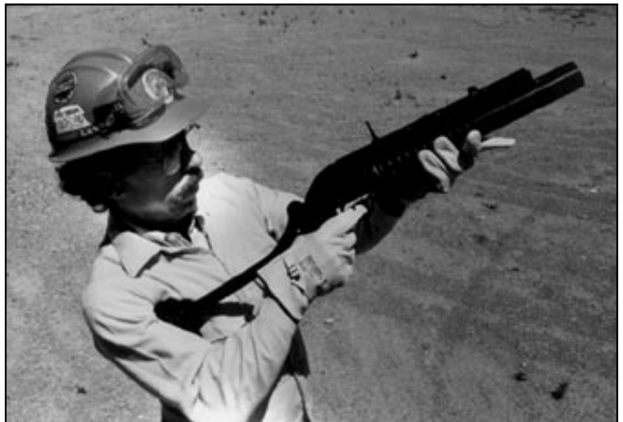
Jim Tour tests flare launchers to determine their suitability for ground ignition.
