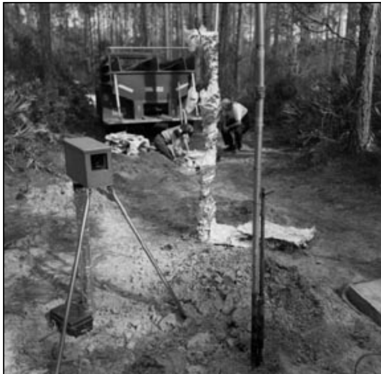
MTDC developed fireproof boxes to protect video cameras used when recording the effects of fire during vehicle entrapments.
