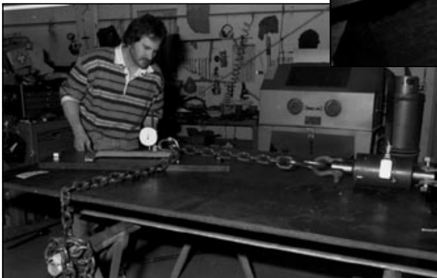
Testing rappel anchor plates for several models of helicopters.
