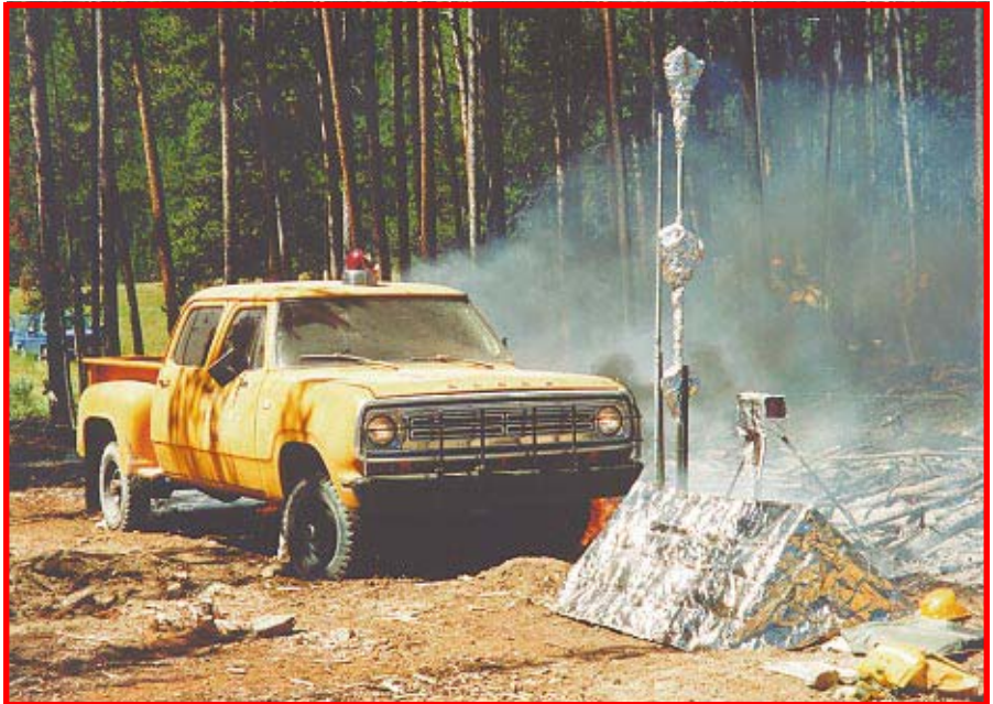
Figure 25—Even after a fire has passed, a vehicle retains heat, acting as a "heat sink."
