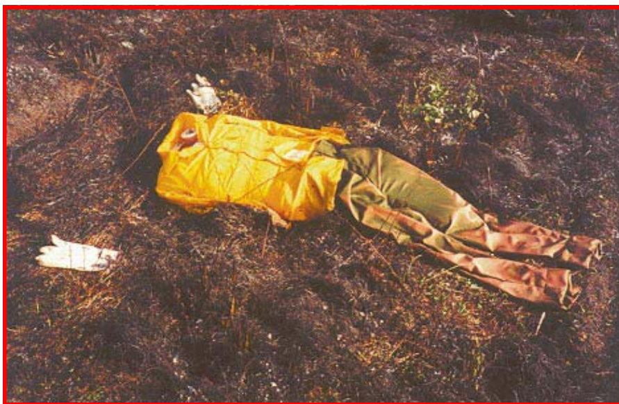
Figure 14—The change in color of the pants shows the effect of heat. Water bags inside the fire shirt and upper pants served as a heat sink, keeping them from becoming as hot as the pant legs.
