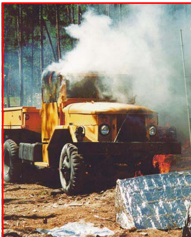
Figure 23—Even though flames did not directly contact the 2½-ton truck, its cab caught fire.
