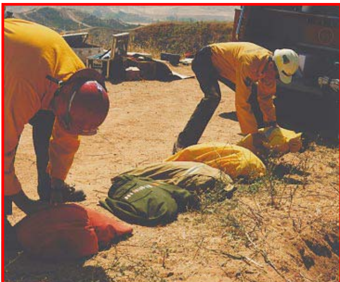
Figure 11—Personal protective clothing was laid out to observe the fire's effects on it.
