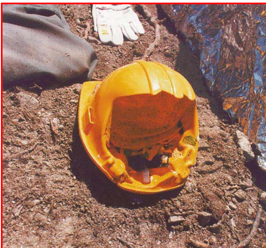
Figure 24—This hardhat shows the difference a few inches can make at ground level. The hardhat melted where it was closest to the fire, but wasn't damaged just a few inches away from the heat.
