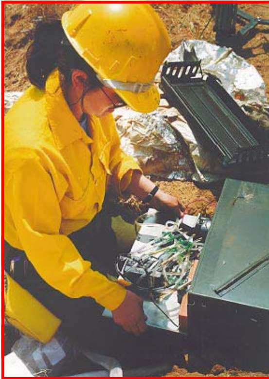
Figures 9 and 10—Gas collection devices sampled gases inside vehicle cabs. Instrumentation was buried inside ammunition boxes so that it would survive the fire.
