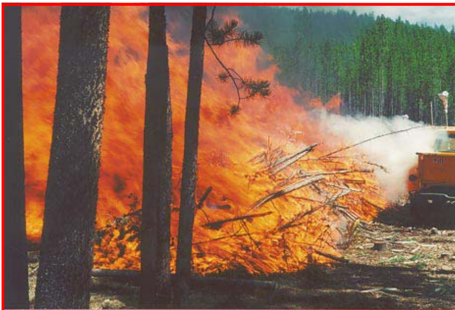
Figure 22—Wind prevented flames from directly contacting vehicles during the test burn near Dillon, MT.
