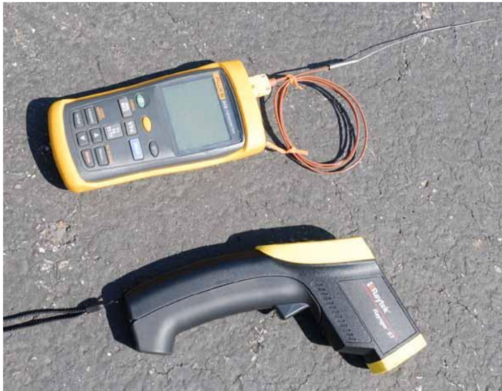
Temperatures were taken using a Type K thermocouple probe (top) and an infrared thermometer (bottom)
