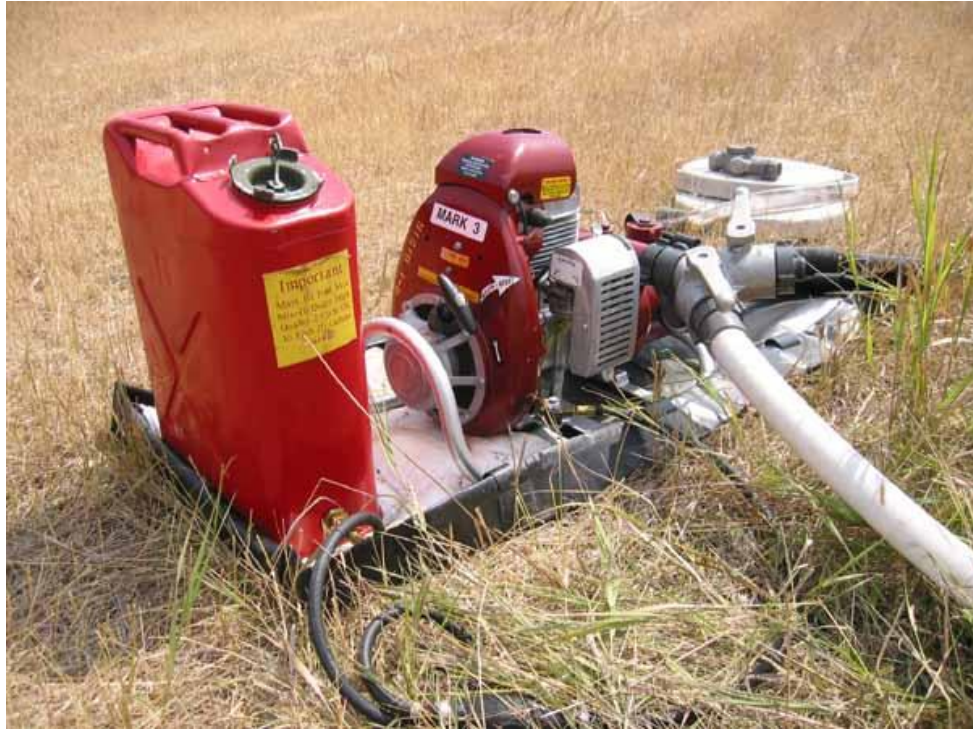
Typical Mark 3 pump and fuel tank installation in a spill containment
