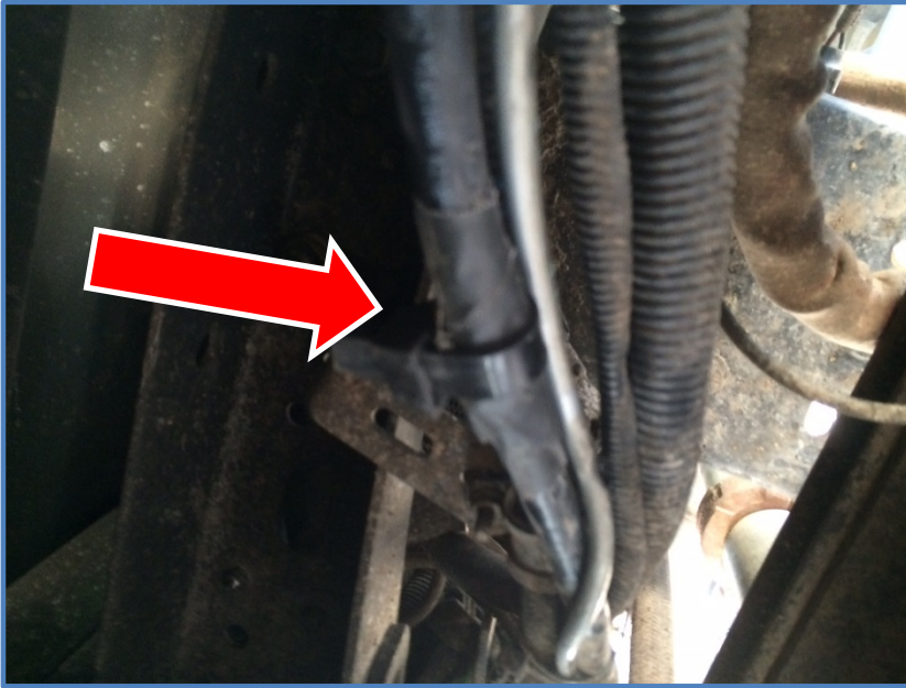
They discovered a hole in the brake air line located approximately three to four feet in front of the right rear axle in the middle of the frame. (Arrow points to where they patched the damaged line with electrical tape and zip tie.)
