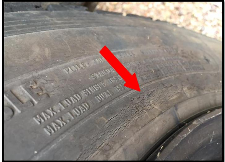
Photo on left shows the tire that triggered this incident had adequate tread depth, but the photo on right also shows the presence of dry cracking.
