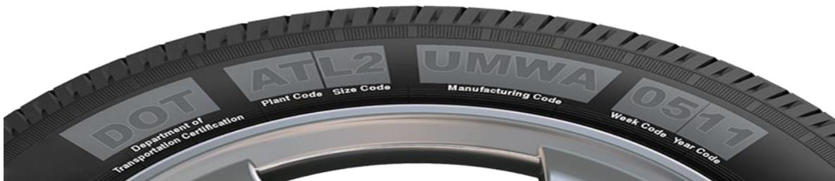
Federal rules mandate that the tire's DOT code be clearly branded or etched on the side of each tire. For most tires, the DOT number is typically 11 digits. **For more information on how to find a tire's DOT Number:**
