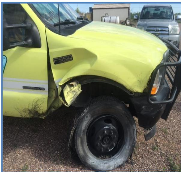
After the crew carrier’s right front quarter panel struck the guardrail two or three times, the vehicle remained in constant contact with the guardrail until it came to a complete stop—approximately 40 feet from the last strike. Once stopped, the driver turned on the hazard lights and exited the vehicle through the driver’s door.
