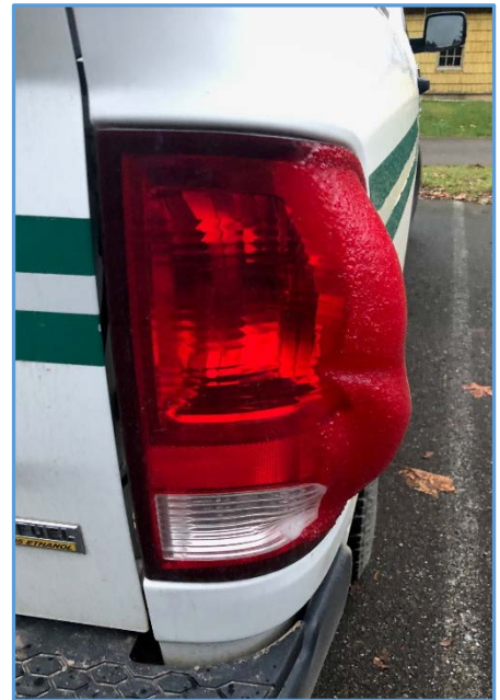
Radiant heat damage to the supervisor's truck.
