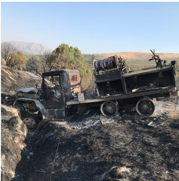
Photo 1. Brush A after burnover, stuck in the gully.
