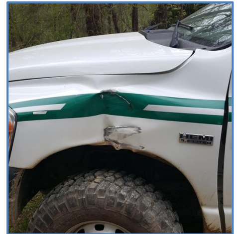
The left front quarter panel of Truck 1 (above) was struck by the left rear portion of Truck 2.
