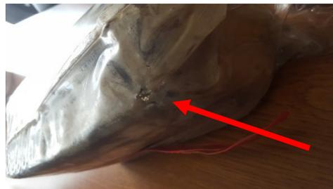
At first glance, the shelter appeared to be in good condition. However once the plastic packaging was removed from the shelter and was unfolded, several areas showed exposed inner-lining as well as signs of delamination.
