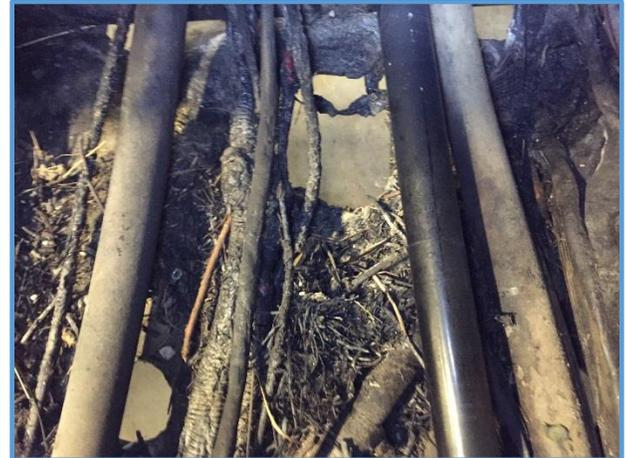
**TOP PHOTO** – Shows the damage to the wiring and gear selector cable caused by the fire that occurred under the UTV's floorboard.
