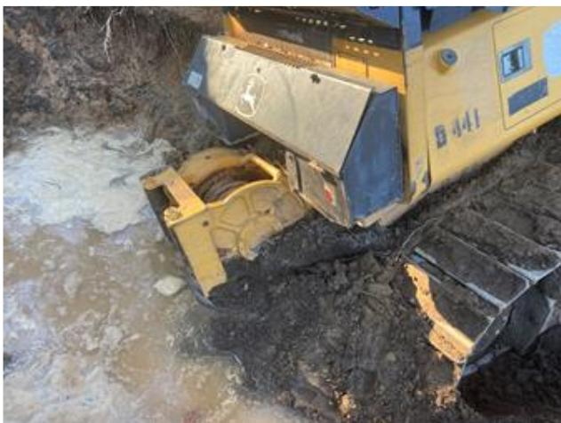
Picture shows the small amount of winch cable to pull, the tight area the swamper was working in, and how the cable was pinned under the track.
