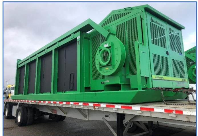
An Air Curtain Burner unit—a new tool that can be used for slash disposal by incident management teams.
