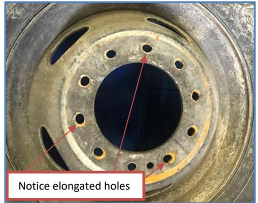
*The inner dual (top photo) and outer dual show the **wallowed-out rim holes**. Look for such wear—it can indicate that the lugs have been overtightened and are damaged.*
