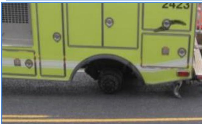
*The Driver's-side rear dual wheels separated from the Engine and traveled across the roadway striking the right front of a passenger vehicle heading north on Hwy 395.*
