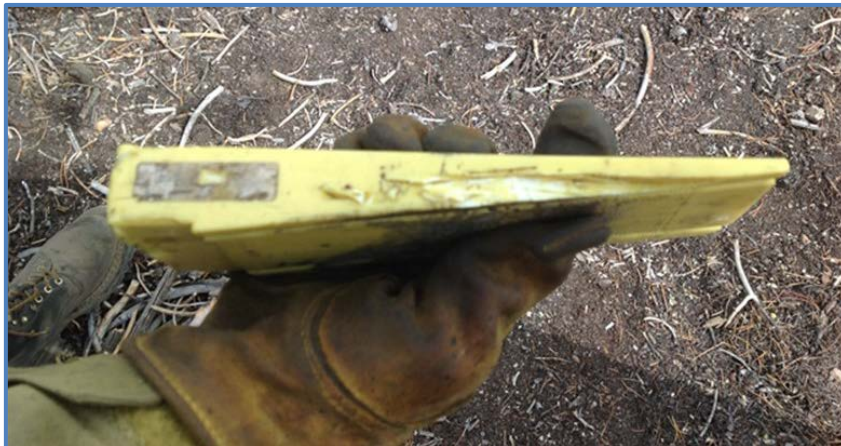
This is the wedge that the sawyer’s saw made contact with causing the kick-back injury during felling operations.
